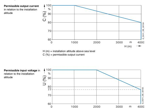
H (m) = installation altitude above sea level U (%) = permissible input voltage
